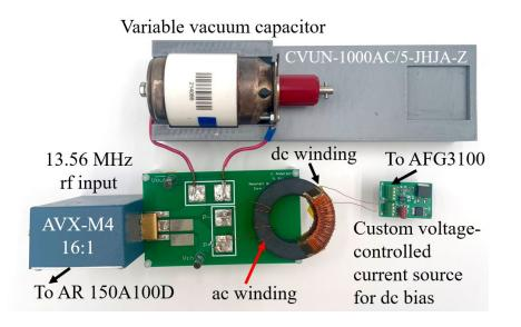
Large signal setup (Using series L and C resonance to calculate core loss and inductance value ) 19
