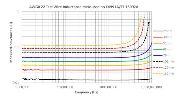
The figures show actual measured inductances and impedances for various wire lengths formed as they would be used for measurements of suppression cores on a typical test set. The test fixture used was an HP16092A with the spring clips extended to maximum width; the test set was calibrated and compensated prior to testing. It can be seen that although the wire inductance is relatively low, the added impedance becomes significant in the high MHz region.
