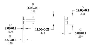
DIMENSIONS **BOLD NUMBERS ARE IN MILLIMETERS**LIGHT NUMBERS ARE IN INCHES
