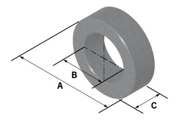
$\begin{array}{ll} \Sigma l/A \ : \ Core\ Constant, \quad l_{_{e}} \ : \ Effective\ Path\ Length, \quad A_{_{e}} \ : \ Effective\ Cross-Sectional\ Area, \quad V_{_{e}} \ : \\ Effective\ Core\ Volume \\ A_{_{L}} \ : \ Inductance\ Factor \end{array}$
