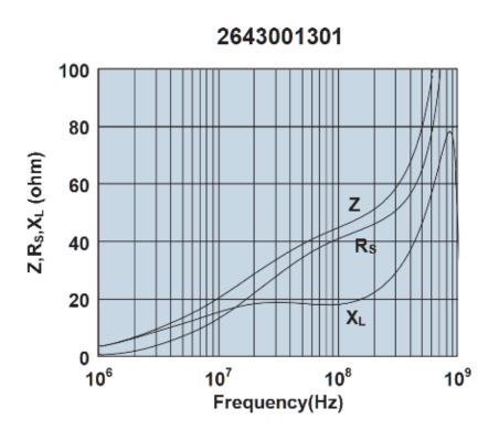
Impedance, reactance, and resistance vs. frequency.
