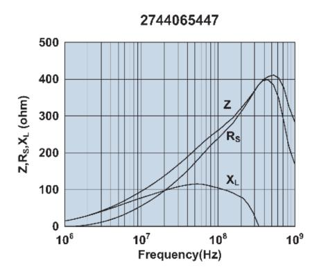
Impedance, reactance, and resistance vs. frequency.
