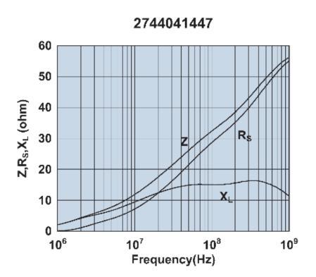
Impedance, reactance, and resistance vs. frequency.
