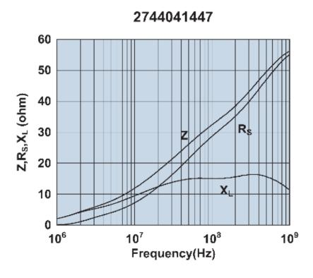
Impedance, reactance, and resistance vs. frequency.
