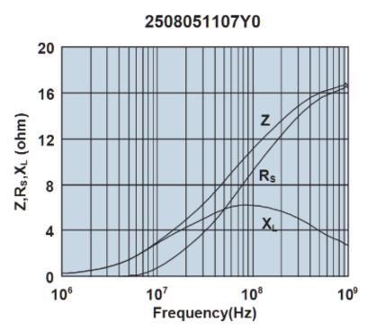
Impedance, reactance, and resistance vs. frequency.
