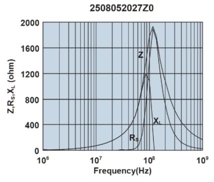
Impedance, reactance, and resistance vs. frequency.
